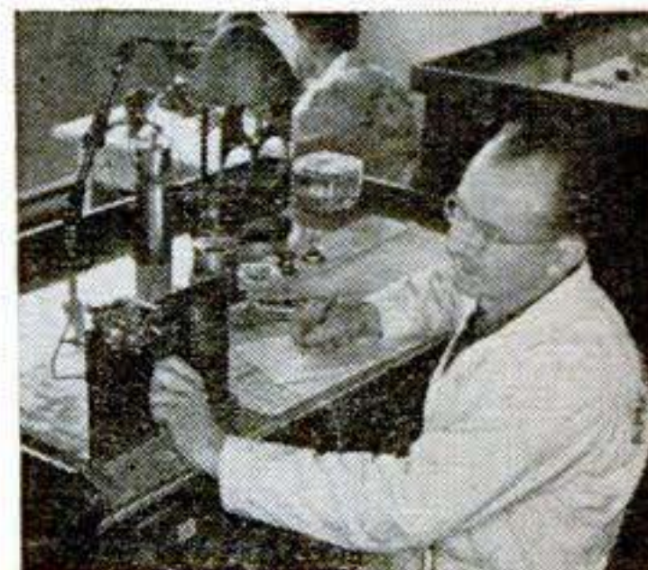
After overhauling a Rate of Climb Indicator, student tests it for proper range deflection, maintaining very rigid tolerances, on a special test unit.
